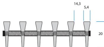
The rolling grilles, which have a free cross section of 72%, are supplied in their standard execution with angle frames with mounting holes in vertical and horizontal flanges. As an alternative the angle frame can be supplied with wall anchors. For mounting in wooden floors the grilles can be supplied in Z-frames. The grilles can be rolled up in order to enable easy convector channel cleaning.
